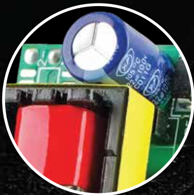
LOW QUALITY CAPACITOR WITH FAKE HOURS PRINTED
